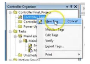
We will create a tag called "Signal\_to\_be\_sent", it is a **Produced** type tag, this will cause the data type to become DINT. Now click the **Connection** button and confirm the entry for Max Consumers is set to 1.
